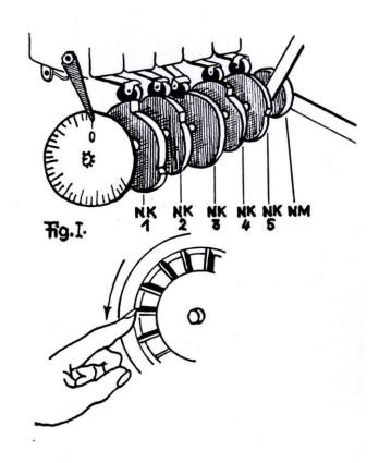
The control of important electrical switching sequences when playing and changing the records is done by the cam contacts NK1 - NK7 (microswitches) attached to the rear of the playing chassis and to the side of the record magazine. The mechanical cam for actuating the tonearm and the sapphire brush, which is called NM in our explanations, is also attached behind the switch NK5.
