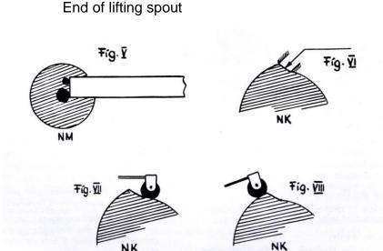
A necessary adjustment of the cam contacts **NK1** to **NK5** is done by adjusting and the shutter cams, the two pressure screws of which must be tightened firmly against the camshaft after the setting has been completed.
