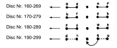
If you would like to expand your vinvl record equipment in this way, you only need to change the bridge connections on the connection strip as shown in the illustration.
