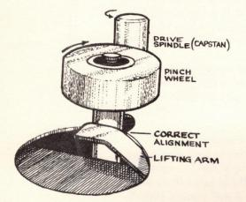
This must be adjusted to give (approx.) 1/32" identation of the pressure wheel on the capstan shaft.
