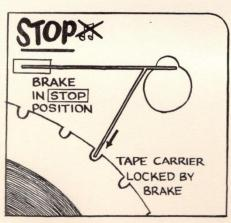
You may first check this operation manually. Since the only purpose of the brake wire is to prevent the spool from rotating, it does not matter if a 'nose' is too large to fit into a slot, provided sufficient tension is present to lock the spool. Make sure that the wire nose is not riding on top of the spool, that it is free to move under its retaining plate and the wire anchorage has not allowed the wire to work free and alter its position relative to the carrier spool slot. (Refer to sketch)
