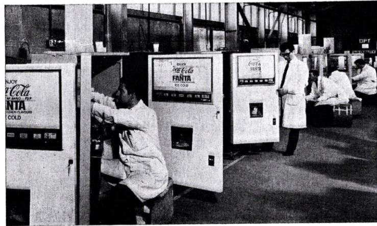
Part of the test line where every machine receives a rigorous inspection before being allowed to leave the factory
